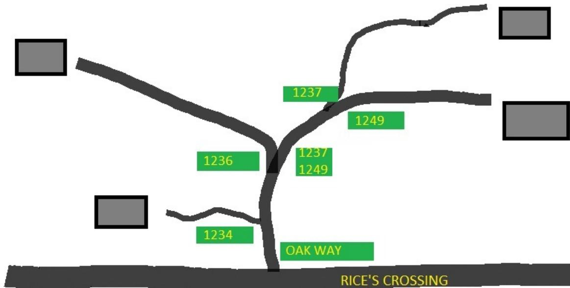
Signs should be of metal and have reflective letters at least 3" tall. If necessary, use arrows to indicate which homes are on each leg. The signs in the picture below are good examples of how to mark a turn leading to multiple homes (note the arrows):
